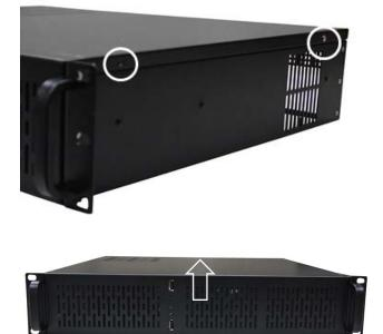
1. Remove the screws from each side of the Chassis. (two on each side)
